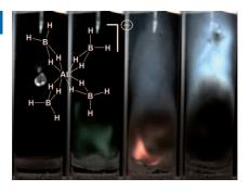
**Lift-off**: The low vapor toxicity of ionic liquids (ILs) make them attractive replacements for hydrazine in rocket fuel. However, ILs will fail to fulfill their revolutionary promise unless toxic oxidizers such as  $HNO_3$  or  $N_2O_4$  can be replaced with safer alternatives such as  $H_2O_2$ . The ILs presented here are hypergolic with  $H_2O_2$  (see picture) and are hydrogen-rich, thus helping to boost performance.
