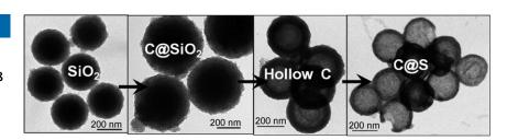
Slowing down the shuttle: C@S nanocomposites (see TEM images) based on mesoporous, hollow carbon capsules were generated by a template-based approach. As the cathode material in a Li-S secondary battery, they display out-
